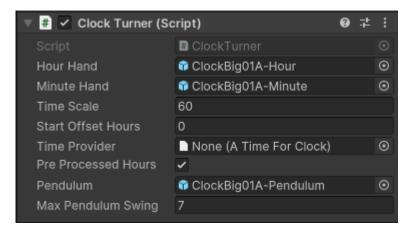
**Hour Hand** and **Minute Hand** are simply the hands of the clock (game objects) which will be rotated around the Z axis to keep time. You must provide a game object for each (not doing so will cause a crash); if you don't want both hands you will need to provide and empty for the absent hand.
